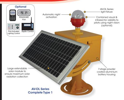
Avlite's low intensity LED obstruction light complete assembly is a self-contained, solar powered obstruction light designed to comply with ICAO LIOL Type A & Type B requirements.
